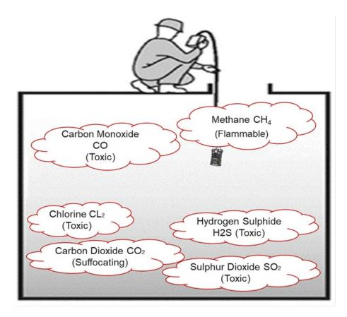
Testing of peak values for a duration of 10 minutes prior to entry is required.
